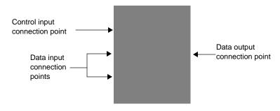
Figure 3-10. Examples of Connection Points
