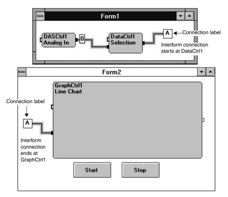
Figure 3-14. Example of Interform Connections
