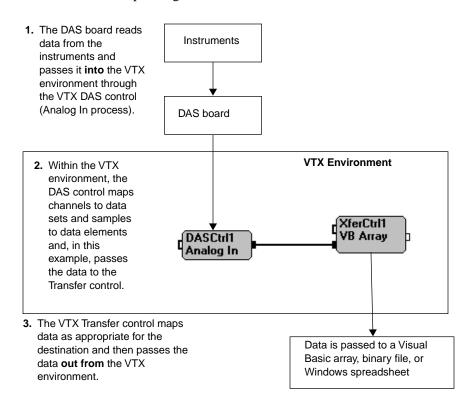
Figure 3-8. Example of Moving Data to and from the VTX Environment
