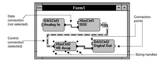
Figure 3-9. Types of Connections
