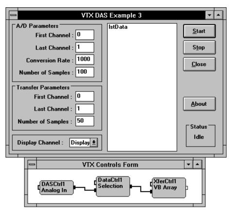
Figure 4-1. Using Separate Forms for a Complex VTX Application
