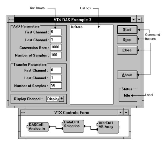
Figure 4-12. Displaying Data in a Visual Basic List Box
