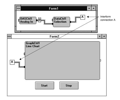
Figure 4-4. Interform Connection Example
