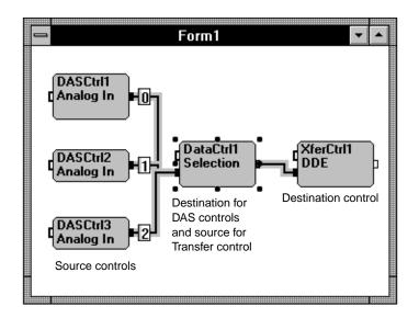
Figure 3-6. Multiple Source Controls to a Single Destination Control
