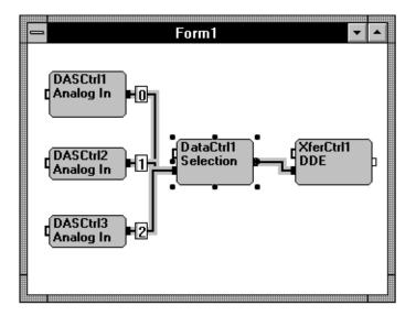
Figure 4-2. Multiple Connections to the Same Input Connection Point
