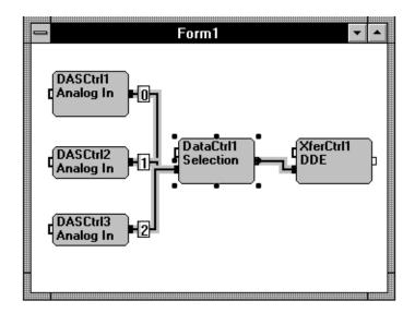
Figure 3-13. Multiple Connections to the Same Connection Point
